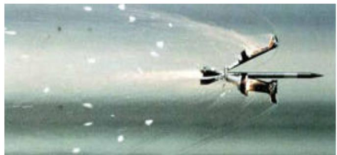
**Figure 6.** Firing a Sabot Fin Round
