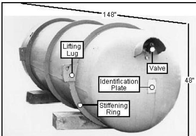
**Figure 1.** Storage cylinder for Uranium Hexafluoride
