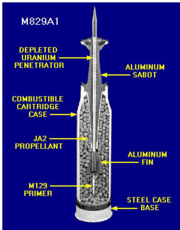
**Figure 5.** Structure of Sabot Fin Round
