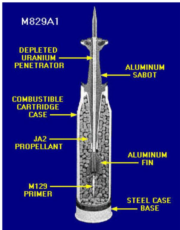
**Figure 5.** Structure of Sabot Fin Round
