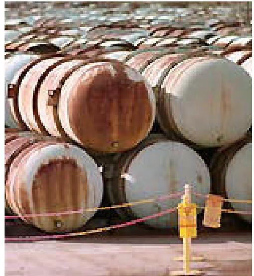
**Figure 2.** Rusting Cylinders stored in the open
