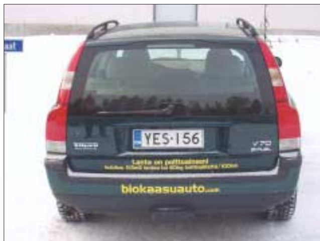
Figure 4: (left) Erkki Kalmari refuelling his vehicle using upgraded biogas. (right) The text on the back of the car says: "Dung is my fuel. Consumption 0.5 m 3 of cow slurry or 50 kg of kitchen waste per 100 km." (Jeremias Kalmari, Jari Jokela)
