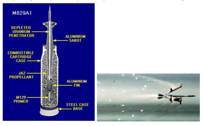
Figure 5. Structure of Sabot Fin Round
