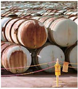
Figure 2. Rusting Cylinders stored in the open
